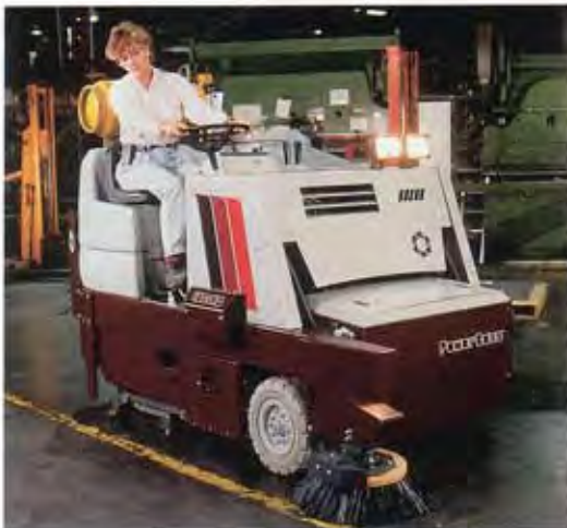
ISS Series.. Dust-controlled, low-dump sweeping with scrubbing
