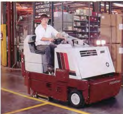
CSS Series.. Pre-sweep, manual dump with scrubbing
